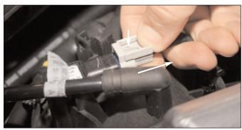
Disconnect the factory connector for the 3-Pin (MAP) sensor. This connector has a locking clip that must be slid back to unlock. Then, squeeze down the locking tab, and push the connector in slightly (toward sensor) and then remove.
