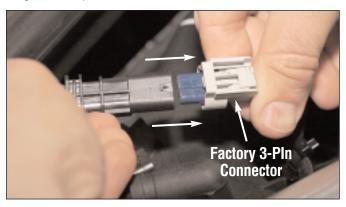
Plug the Interceptor harness connector into the factory 3-Pin MAP sensor wiring harness connector. NOTE: The correct orientation of the connector is shown above.
