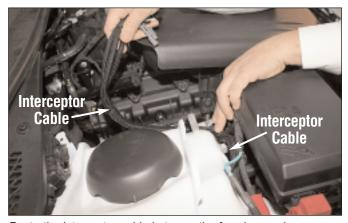
Route the Interceptor cable between the fuse box and passenger side strut tower.
