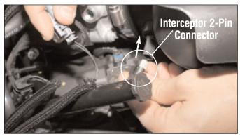
Route the Interceptor harness and plug the Interceptor 2-Pin connector into the vehicle intake air temp sensor. **NOTE: The correct orientation of the connector is shown above.**
