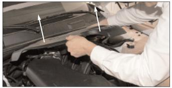
CAREFULLY lift off the engine cover to avoid scratching it on surrounding surfaces and place it to the side while installing the Hypertech Interceptor.
