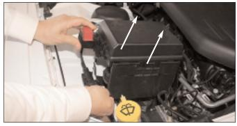
Locate fuse box in the engine compartment on the passenger side. Press the locking tabs to disengage fuse box and lift up to expose empty compartment. Locking tabs may vary slightly from those shown above.
