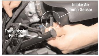
Disconnect the factory connector from the 2-Pin (intake air temp) sensor.
