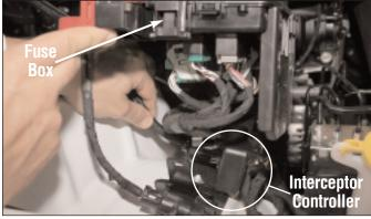
Place Interceptor Controller on its side in the compartment, making sure no cables are pinched or bent. Then re-install the fuse box back to its original location.
