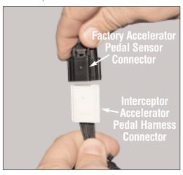
Plug the Interceptor accelerator pedal harness connector into the vehicle's factory accelerator pedal sensor connector.
